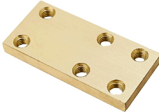
The Long D Plate (Part # 80329002) is made of brass and fastened to the back of a multi-cylinder SD Series Type D interlock to allow front mounting (see SD Series Data Sheet 1.4). The thickness of the Long D Plate is 3/8". To order this plate with your multi-cylinder SD Series Type D interlock, put the letter "P" in column fourteen of the interlock part number - reference the SD Series Ordering Guide.
