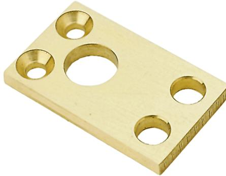
The FN Plate (Part # 155987001) is made of brass and fastened to the end of a SD Series Type FN interlock to allow alternative mounting scenarios (see SD Series Data Sheet 1.7). The thickness of the FN Plate is 1/4". To order this plate with your SD Series Type FN interlock, put the letter "P" in column fourteen of the interlock part number - reference the SD Series Ordering Guide. The plate (when ordered) will be bolted to your Type FN interlock.
